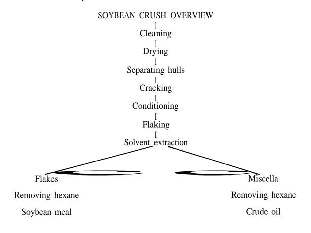
The quality of the soybean meal is most affected by the quality of the raw soybeans and by the process of removing the hexane. Before discussing the quality parameters, I want to discuss the process of hexane removal. The equipment which is used is called a desolventizer toaster; industry jargon shortens this to DT (Fig. 2).
