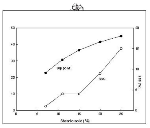
**Figure 1.** Effect of stearic acid content on fat composition (content of tri-saturated triacylglycerol) and slip points. SSS = tri-saturated triacylglycerol.
