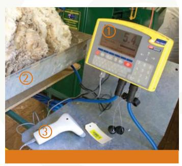
Image 1. Tru-Test indicator and barcode scanner
