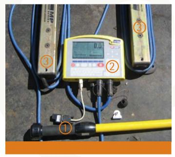
Image 9. Tru-Test indicator, stick reader and weigh bars
