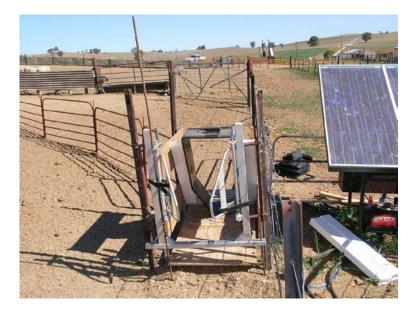
There were numerous "teething" problems when the platform was first put in. The RFID read range was very poor, apparently from some sort of interference inhibiting the effectiveness of the reader. Originally a set of Allflex rubberised flap readers were used, with the animals tagged with FDX-B tags. More than 50% of the tags were not being read, so the reader was changed for an Allflex portal reader. This partially solved the read problems, but as can be seen from the above photo, if the setup
