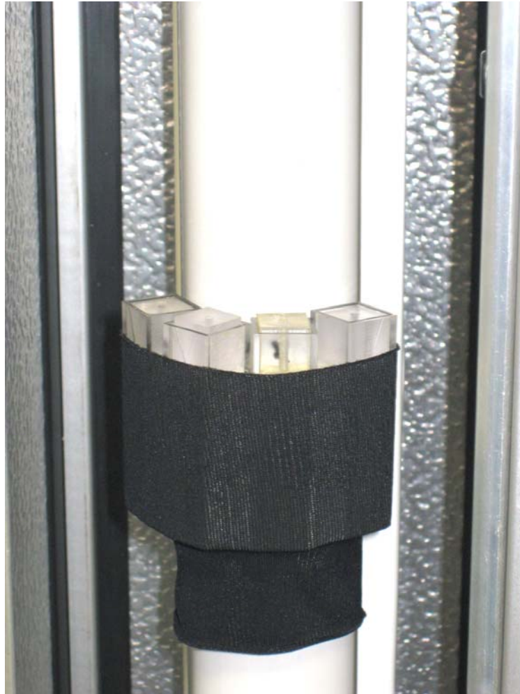
Figure 4 Sample cuvettes mounted against the UVB tube.
