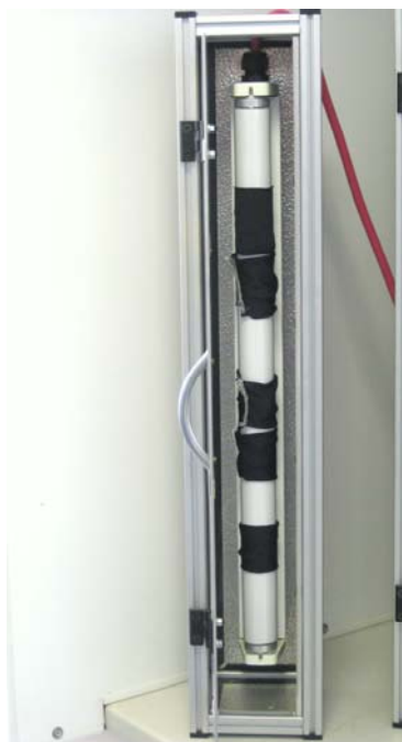
Figure 3 UVB lightbox housing Philips TL20W/12RS (UVB) tube. Five black elastic fabric sleeves for holding sample cuvettes in contact with the tube are shown.
