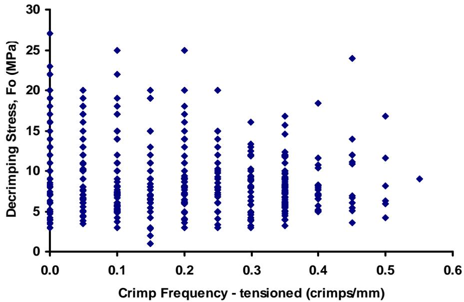
Figure 10: Relationship between crimp frequency (tensioned) and decrimping force ( $F_0$ ). Pooled data from all fibres from all sheep ( $n_{\text{fibres}} = 678$ )
