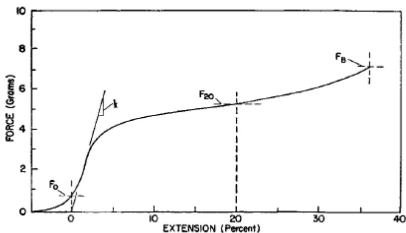
**Figure 7: Typical force extension curve for a wool fibre (Evans, 1954)**
