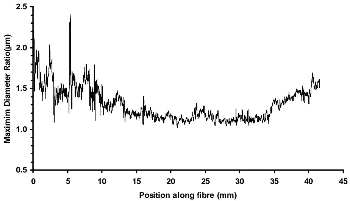
Figure 17: Maximum diameter ratio (ellipticity) of nominal 10 micron wire obtained from SIFAN 3 at an orientation of 60 degrees and 150 degrees.
