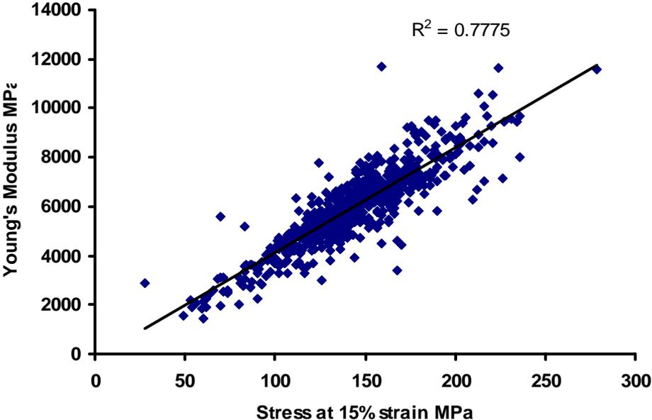
Figure 13: Young's modulus in relation to stress at 15% strain ( $F_{15}$ ). Pooled data from all fibres from all sheep ( $n_{\text{fibres}} = 678$ )
