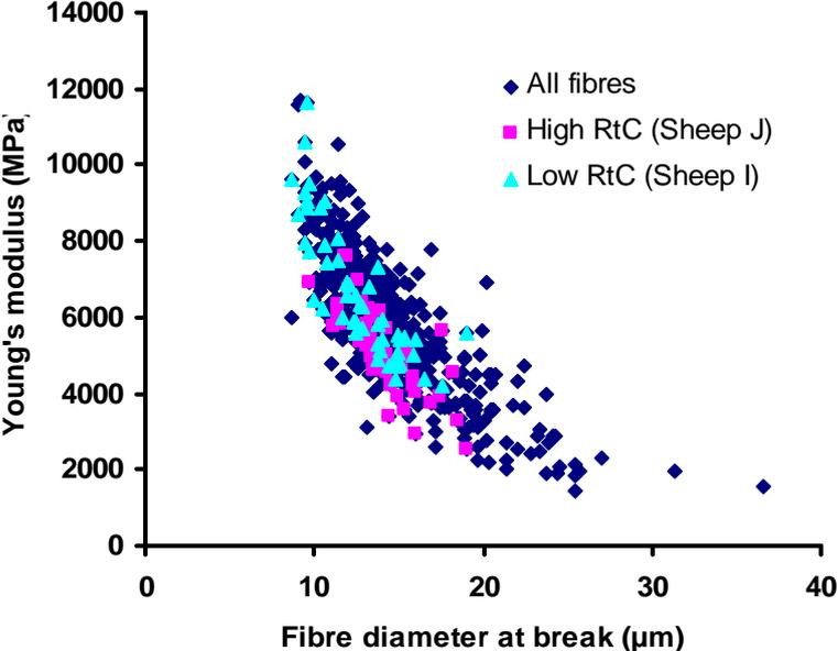
Figure 4 The effect of RtC on the diameter dependency of Young's Modulus
