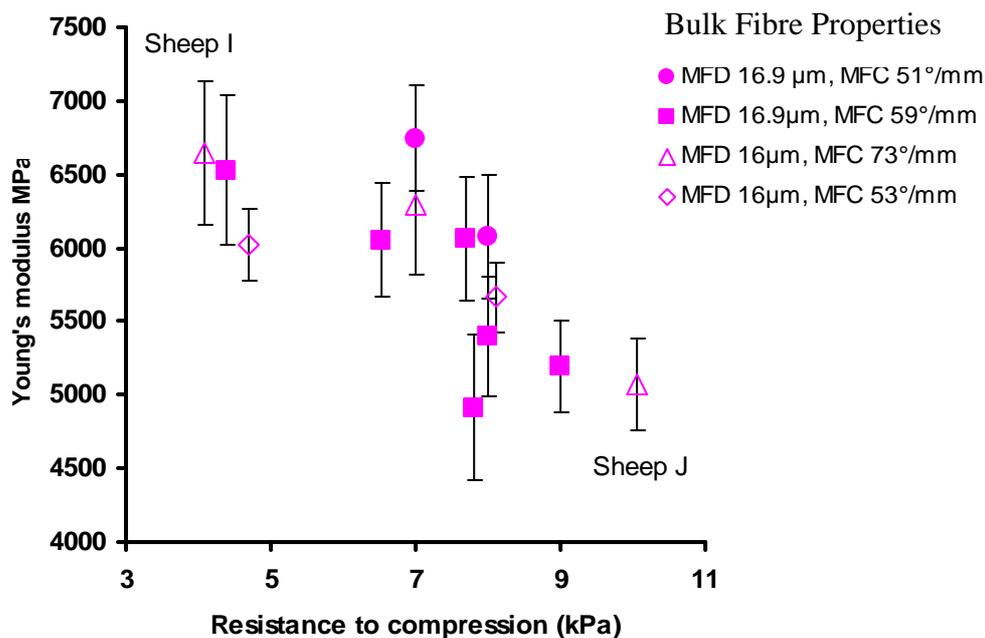
**Figure 6: The relationship between Young's modulus and resistance to compression (RtC) showing the 95% confidence interval**
