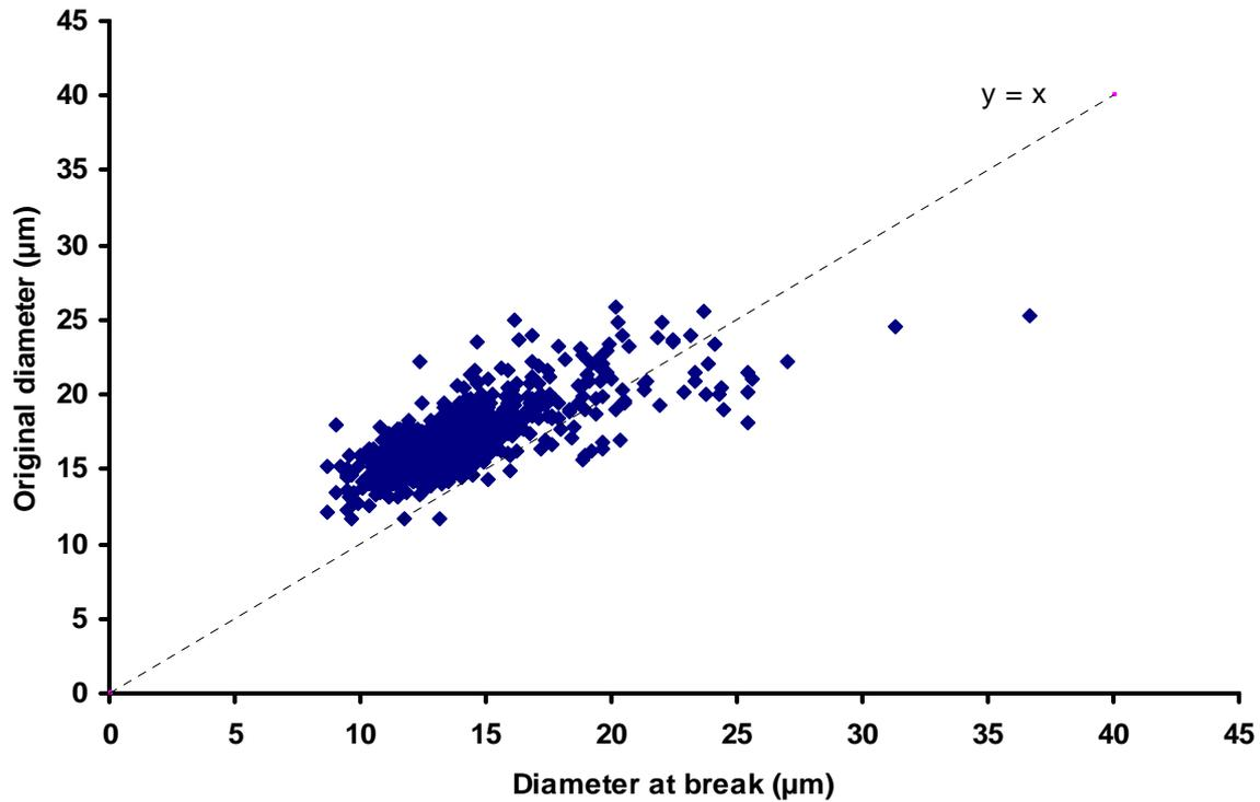
**Figure 3: Relationship between original fibre diameter (vibroscope) and diameter at the break (optical microscope). Pooled data from all fibres from all sheep ( $n_{\text{fibres}} = 678$ )**
