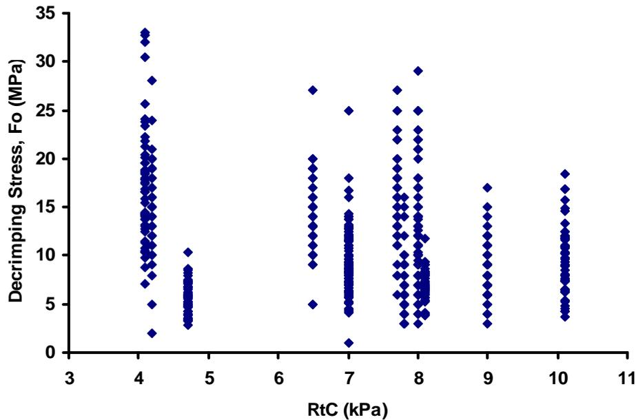
**Figure 12: Relationship between RtC and decrimping force ( $F_0$ ). Pooled data from all fibres from all sheep ( $n_{\text{fibres}} = 678$ )**
