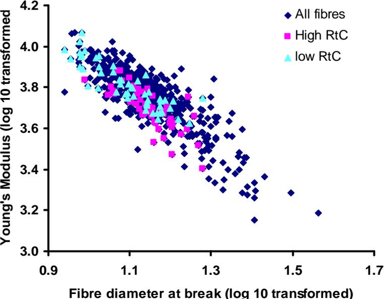
Figure 5 The effect of RtC on the diameter dependency of Young's Modulus where all data is log<sub>10</sub> transformed.
