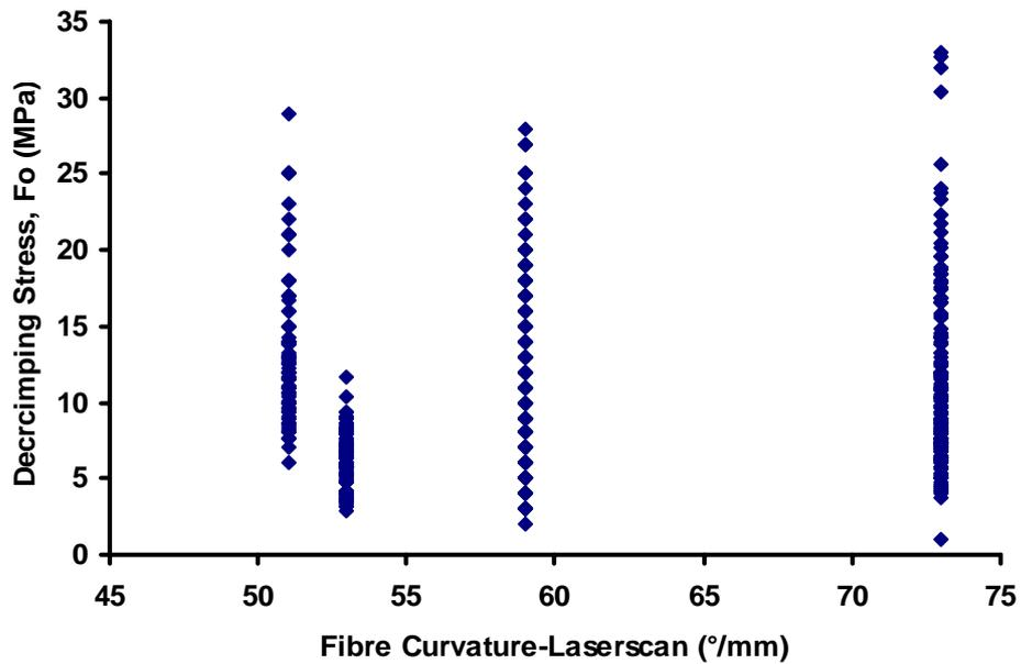
Figure 11: Relationship between Laserscan fibre curvature and decrimping force ( $F_0$ ). Pooled data from all fibres from all sheep ( $n_{\text{fibres}} = 678$ )
