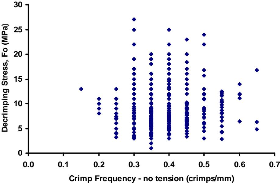
Figure 9: Relationship between crimp frequency (no tension) and decrimping force ( $F_0$ ). Pooled data from all fibres from all sheep ( $n_{\text{fibres}} = 678$ )
