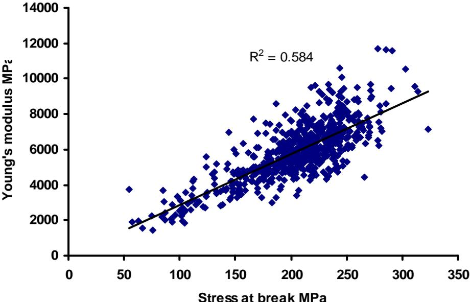
Figure 14: Young's modulus in relation to stress at break. Pooled data from all fibres from all sheep ( $n_{\text{fibres}} = 678$ )
