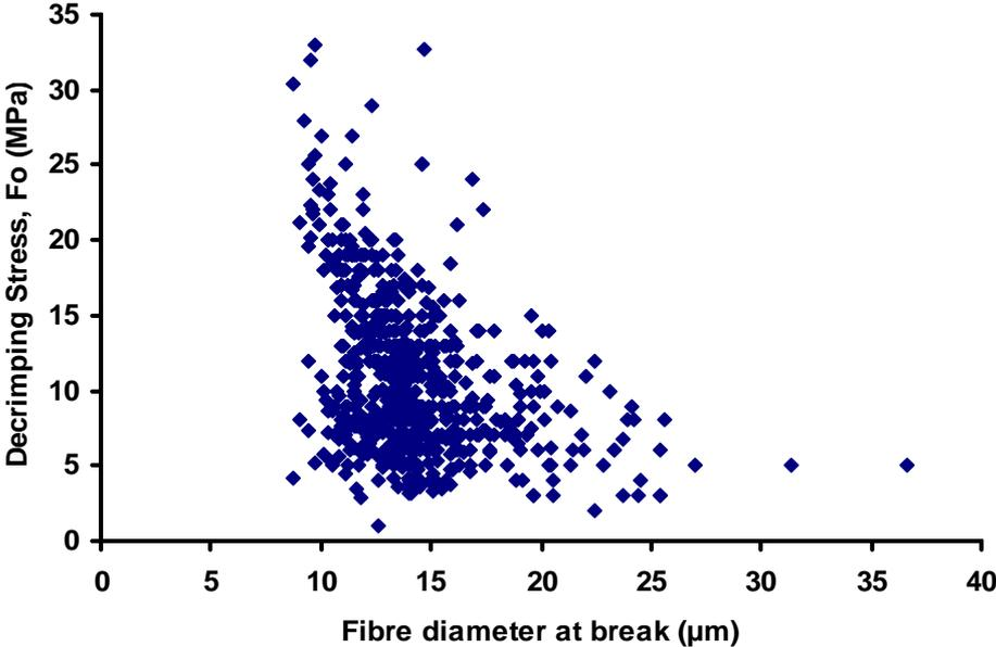
Figure 8: Relationship between fibre diameter at the break and decrimping force ( $F_0$ ). Pooled data from all fibres from all sheep ( $n_{\text{fibres}} = 678$ )
