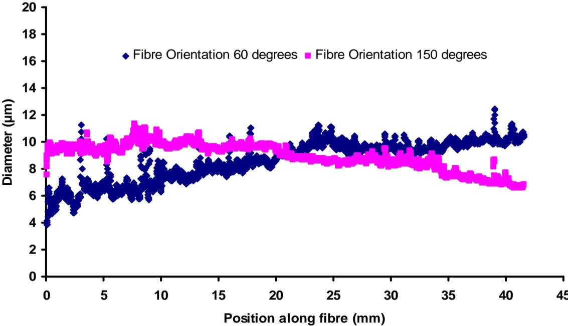
Figure 16: Orthogonal diameter profile of nominal 10 micron wire obtained from SIFAN 3 at an orientation of 60 degrees and 150 degrees.
