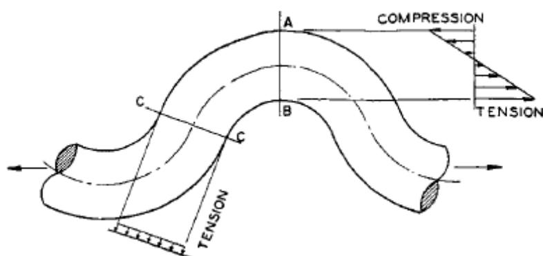
**Figure 1 Stress in a crimped wool fibre under small tension (Evans, 1954)**
