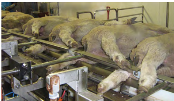
Figure 3. High frequency immobilization (charge coming from back bar, with water used for better contact).
