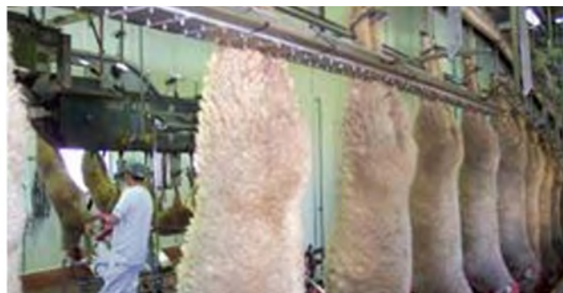
Figure 4. Low voltage pre-dressing system (current applied through rail to hocks).
