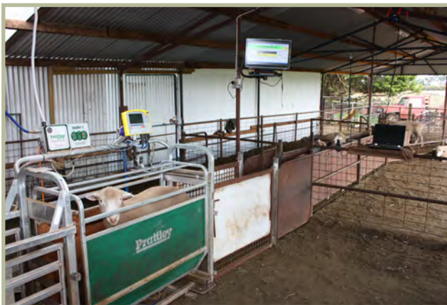
ABOVE: Autodrafting using Prattley autodrafter and Tru-test XR3000 indicator and large screen display
