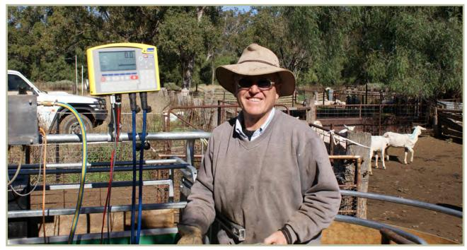
ABOVE: Ray Haigh autoweighing and drafting using a Tru-test XR3000 indicator and Prattley 3-way autodrafter
