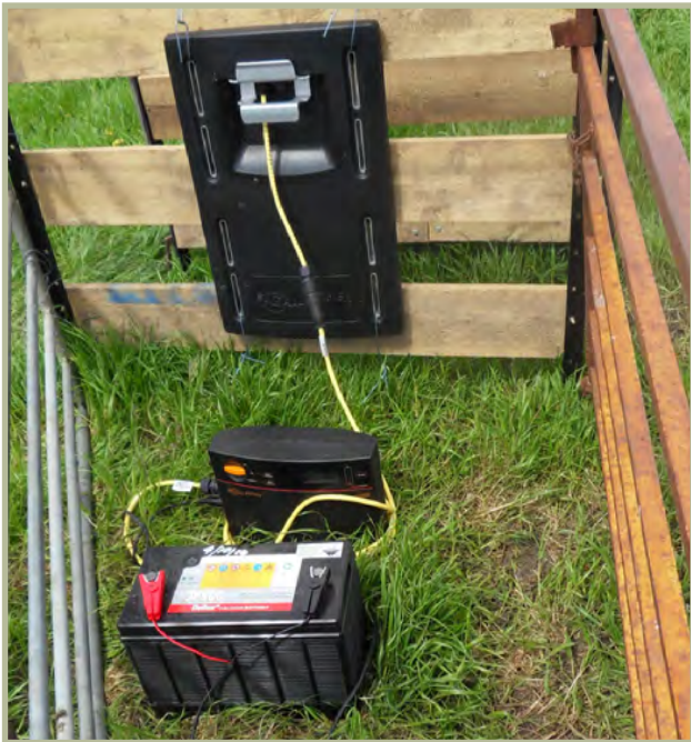
ABOVE: Reading e-ID tags with a Gallagher panel reader for Pedigree Match Maker
