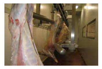
**Figure 4**. Post-dressing medium voltage electrical stimulation unit, bottom rail is active. Source: K. L. Pearce.
