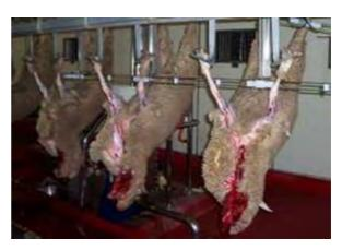
**Figure 2.** Suspended sheep carcase showing the Y-cut and the electrodes in contact with the front legs. Source: E.S. Toohey.
