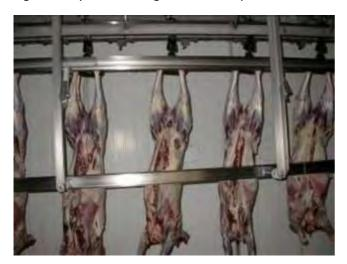
**Figure 3**. High voltage electrical stimulation unit, bottom rail is active. Source: E.S. Toohey.
