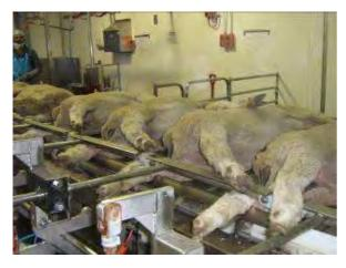
**Figure 1**. High frequency immobilisation used immediately post exsanguination and before the carcasses are placed on the chain. Source: E.S. Toohey
