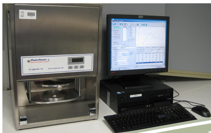
Phabrometer handle meter with special CRC software for knitted fabric". Image courtesy of AWTA.
