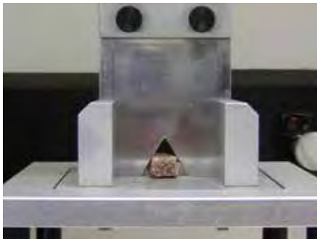
Measurement of shear force on cooked meat.
