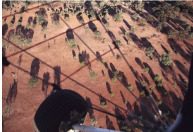
Figure 2. Observer's view of transect from the Drifter ultralight. Kangaroos are recorded by species and distance from the aircraft as guided by the grid wires. At 50 knots, the ultralight emulates the use of a helicopter but at a much lower cost.
